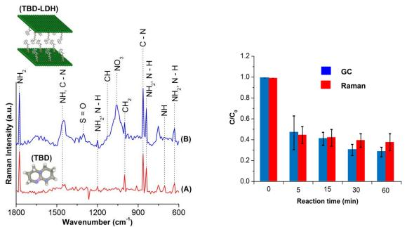
Figure 3 (left) Raman spectra of (A) TBD and (B) TBD-LDH detected with a Perkin Elmer 785 nm Raman spectrometer, and (right) Concentration of triglyceride oil using DMC as methylating agent and  $T_{rxn} = 70$  °C.
