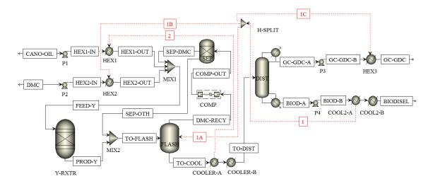
Fig. 1. Process flow diagram using Aspen Plus simulation for a glycerol-free biofuel production facility. The red dotted lines indicate heat integration techniques that reduce overall energy input. This process is 15% more energy efficient than current biodiesel production facilities. http://dx.doi.org/10.1016/j.fuproc.2013.03.030
